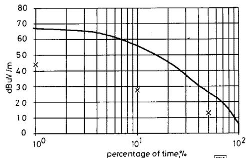
Fig. 1 Cumulative frequency distribution for entire database of measurements and comparison with ITU-R predictions (X)
