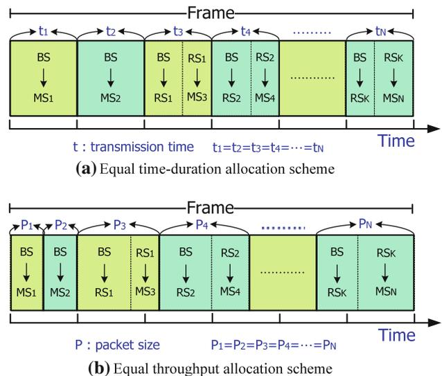
**Fig. 3** Frame structure for the equal time-duration and equal user-throughput allocation schemes with  $N$  users. (a) Equal time-duration allocation scheme: each user can send data in one slot of each frame. (b) Equal user-throughput allocation scheme: each user can send a packet with size  $P$  in each frame
