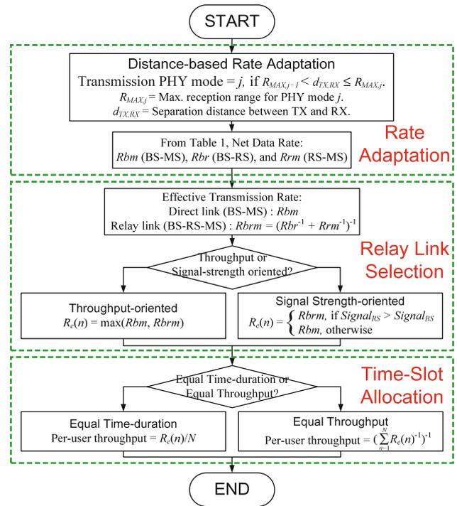
Fig. 2 Procedures of the resource allocation for a user, including three steps: (1) rate adaptation, (2) relay link selection, and (3) time-slot allocation
