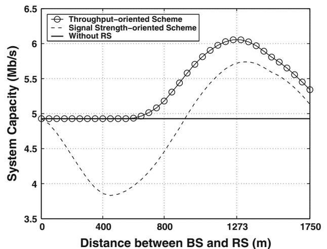
**Fig. 4** Achieved system capacity for different relay selection rules, where the equal time-duration allocation scheme is used
