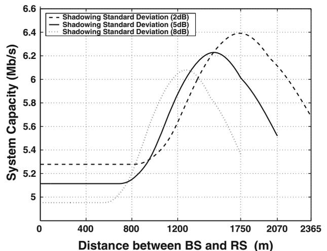
**Fig. 10** System capacity versus relay location for various shadowing standard deviation  $\sigma$ , using the throughput-oriented selection scheme and the equal time-duration allocation scheme
