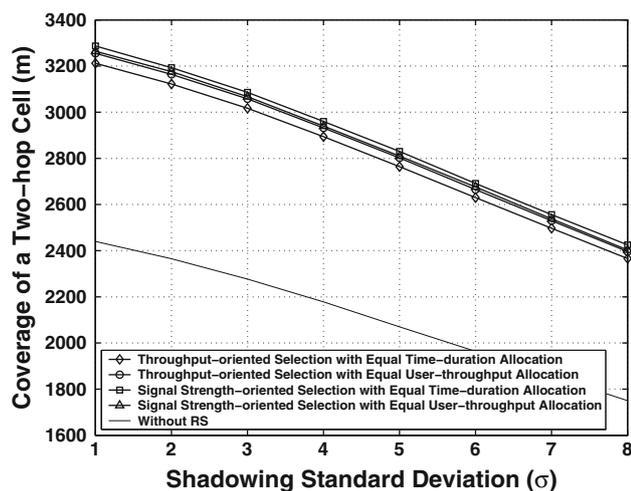
**Fig. 11** Coverage of a two-hop cell for various shadowing standard deviation  $\sigma$ , where 8 RSs are deployed at the optimal locations and the outage probability requirement is  $P_{o,req} = 0.1$
