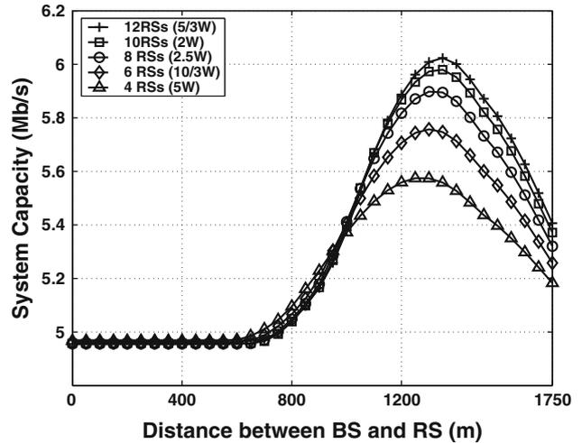
**Fig. 9** Achieved system capacity and optimal relay location for different number of deployed RSs, where the total transmission power of RSs is fixed at 20 W
