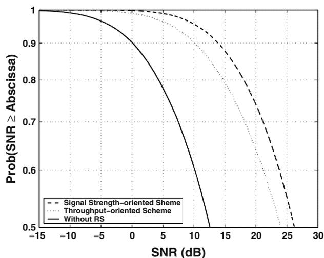
**Fig. 7** The complementary CDF of users' SNR according to various relay selection rules, where the equal time-duration allocation scheme is used and the RSs are deployed at the optimal locations
