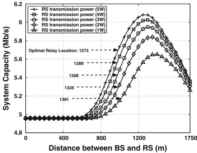
**Fig. 8** Achieved system capacity and optimal relay location for various relay transmission power, where there are 8 RSs in a cell
