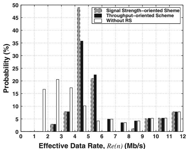
**Fig. 6** The PMF of effective data rate  $R_e(n)$  according to different relay selection rules, where the equal time-duration allocation scheme is used and the RSs are deployed at the optimal locations
