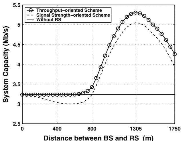
**Fig. 5** Achieved system capacity for different relay selection rules, where the equal user-throughput allocation scheme is used
