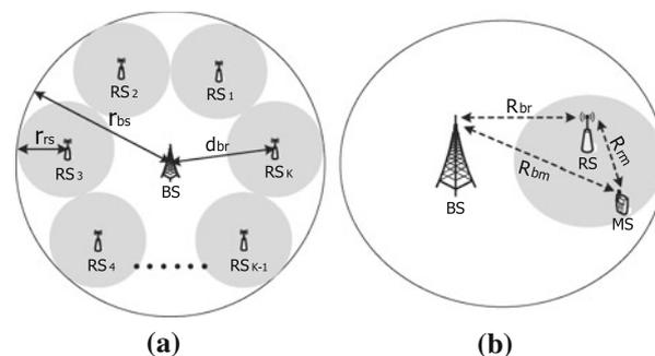
**Fig. 1** The architecture of a two-hop relaying network with one BS and  $K$  RSs. **a** A two-hop relay network. **b** Transmission rate between transmitter and receiver
