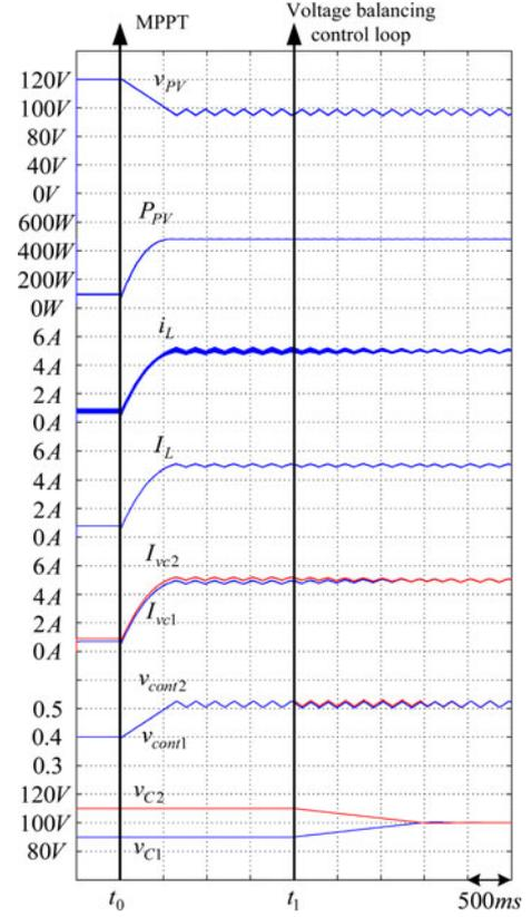
Fig. 8. Simulated results for the proposed MPPT and voltage balancing control methods.
