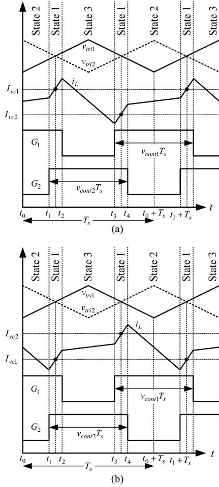
Fig. 6. The illustrated waveforms for the case of  $v_{\text{cont1}} + v_{\text{cont2}} > 1$ : (a) when  $v_{C1} > v_{PV} > v_{C2}$ ; (b) when  $v_{C2} > v_{PV} > v_{C1}$ .
