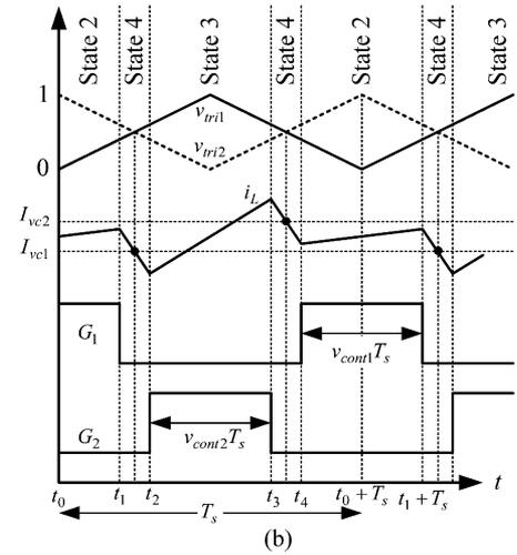
Fig. 5. Illustrated waveforms for the case of  $v_{cont1} + v_{cont2} < 1$ : (a) when  $v_{PV} > v_{C1} > v_{C2}$ ; (b) when  $v_{PV} > v_{C2} > v_{C1}$ .
