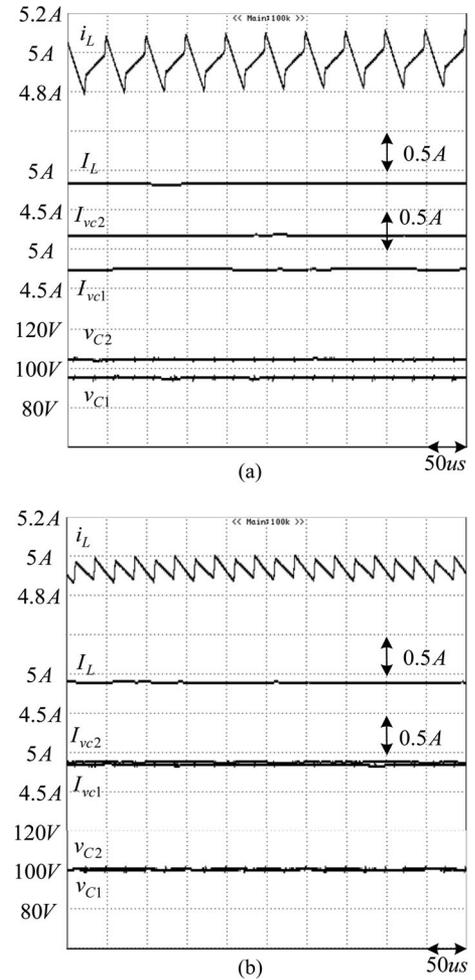
Fig. 10. Enlarged steady-state waveforms (a) before the voltage balancing control loop is applied and (b) after the voltage balancing control loop is applied.
