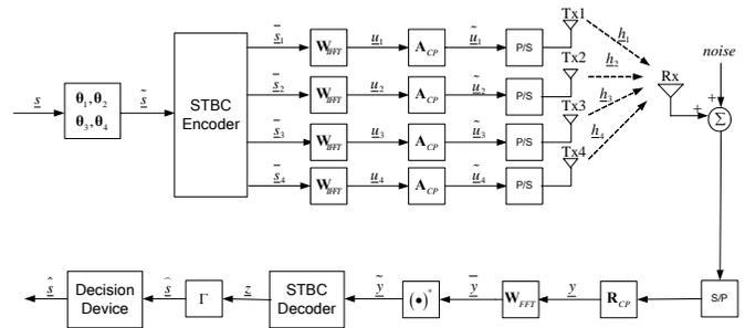
**Fig. 1.** Four-transmit-antenna STBC OFDM transceiver model with block precoders
