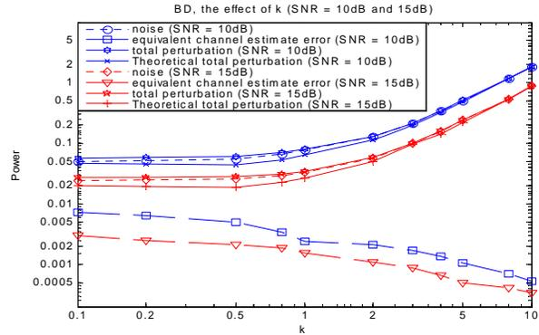
Fig. 8. Theoretical and simulated total perturbation powers
