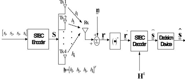
Fig. 2. Basic STBC transceiver model in frequency domain
