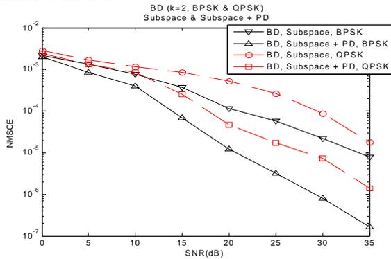
Fig. 6. Improved performances by the phase-direct technique
