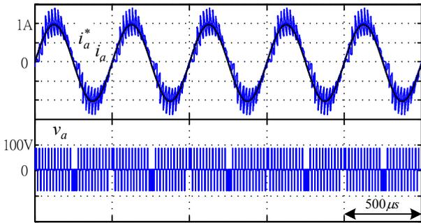
Fig. 9. Simulation results of PMEDS fed by full-bridge circuit with dead-time compensation loop at 2kHz/1A.
