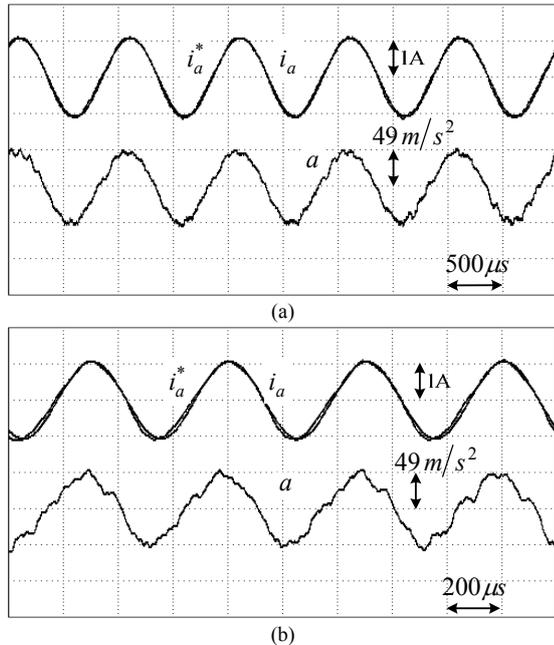
Fig. 11. Experimental results with only feedback loop and dead-time compensation loop: (a) 1kHz/1A; (b) 2kHz/1A.
