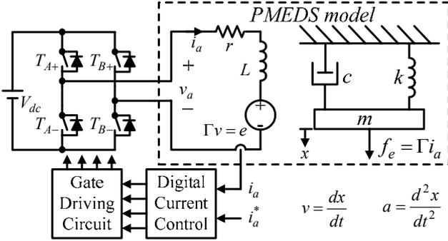
Fig. 2. System configuration and PMEDS model.
