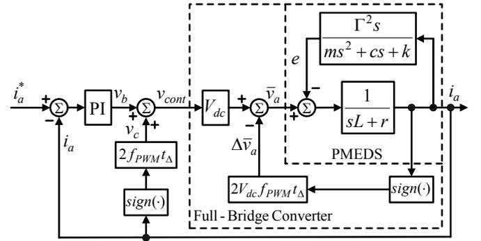
Fig. 5. Proposed current control for PMEDS.
