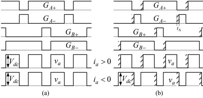
Fig. 4. Gate signals and the resulting armature voltage  $v_a$ :
