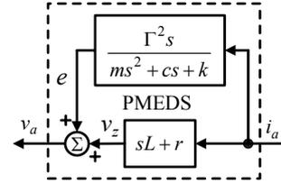
Fig. 7. Equivalent block diagram for PMEDS
