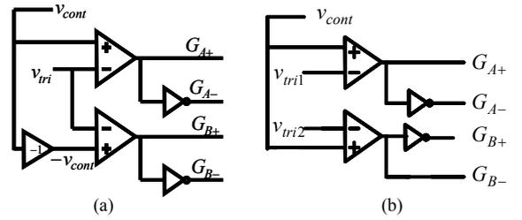
Fig. 3. (a) Single-carrier unipolar switching scheme; (b) multi-carrier unipolar switching scheme.
