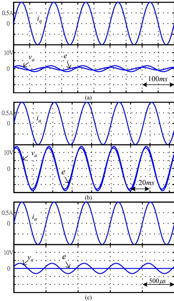
Fig. 6. Simulation results of PMEDS fed by ideal current source: (a) 10Hz/1A; (b) 30Hz/1A; (c) 2kHz/1A.
