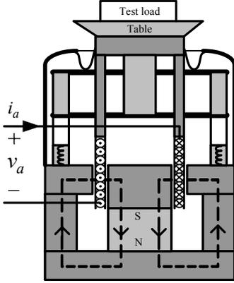
Fig. 1. Permanent-magnet electrodynamic shaker (PMEDS).
