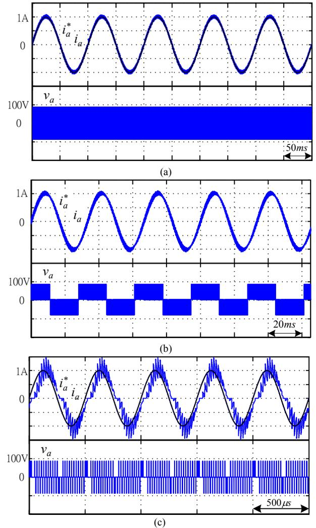
Fig. 8. Simulation results of PMEDS fed by full-bridge circuit : (a)10Hz/1A; (b)30Hz/1A; (c)2kHz/1A.
