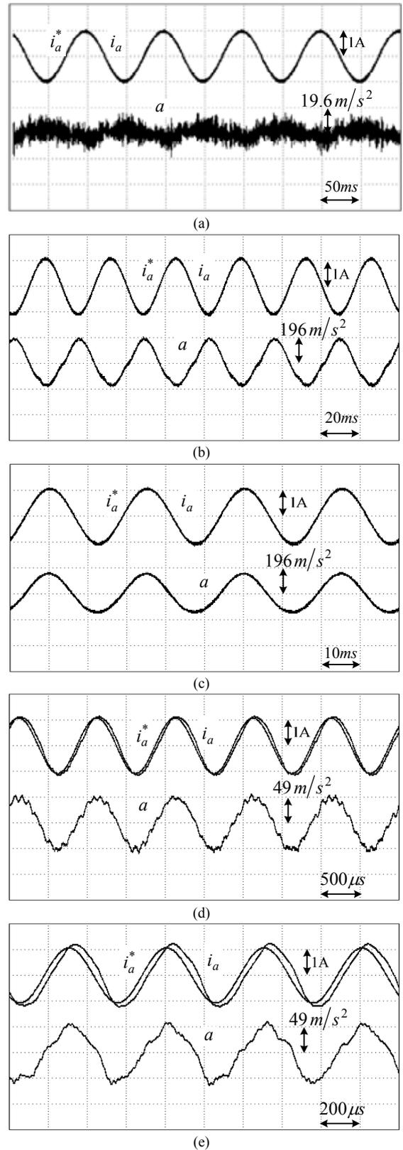
Fig. 10. Experimental results with only feedback loop: (a) 10Hz/1A; (b) 30Hz/1A; (c) 40Hz/1A; (d) 1kHz/1A; (e) 2kHz/1A.
