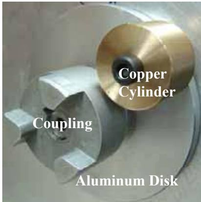
Fig. 2. Experimental position-dependent load.
