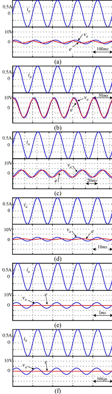
Fig. 4. Simulation results of PMEDS (0.311kg) fed by an ideal current source: (a) 10Hz/1A; (b) 20Hz/1A; (c) 30Hz/1A; (d) 100Hz/1A; (e) 1kHz/1A; (f) 2kHz/1A.
