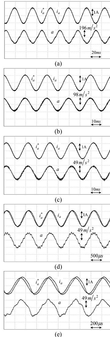
Fig. 11. No-load experimental results with only feedback loop: (a) 30Hz/1A; (b) 50Hz/1A; (c) 250Hz/1A; (d) 1kHz/1A; (e) 2kHz/1A.
