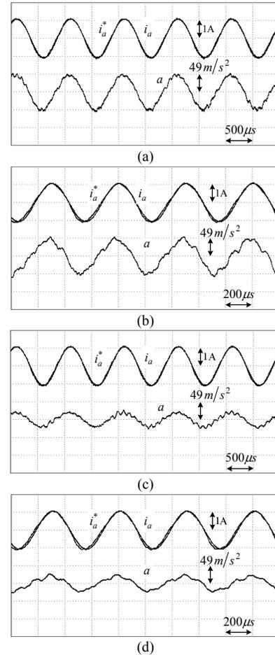
Fig. 13. Experimental results with PI feedback loop and dead-time compensation loop, (a)  $1kHz/1A$  (no load); (b)  $2kHz/1A$  (no load), (c)  $1kHz/1A$  (load  $0.311kg$ ); (d)  $2kHz/1A$  (load  $0.311kg$ ).
