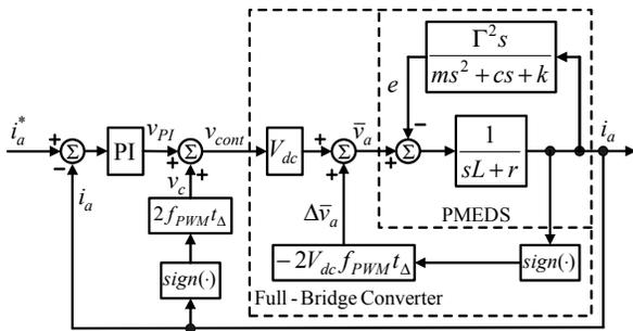
Fig. 7. Proposed current control for PMEDS.
