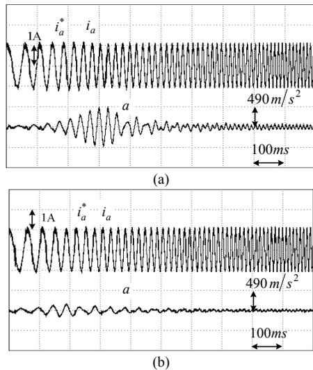
Fig. 14. Measured waveforms with sweeping command frequency (a) with no load; (b) with load 0.311kg.
