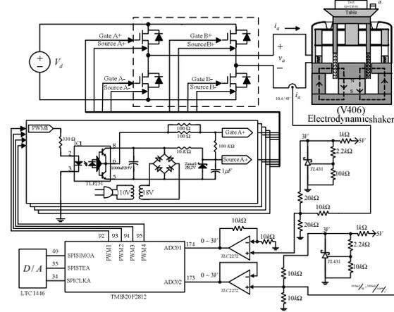
Fig. 10. The DSP-based experimental system.
