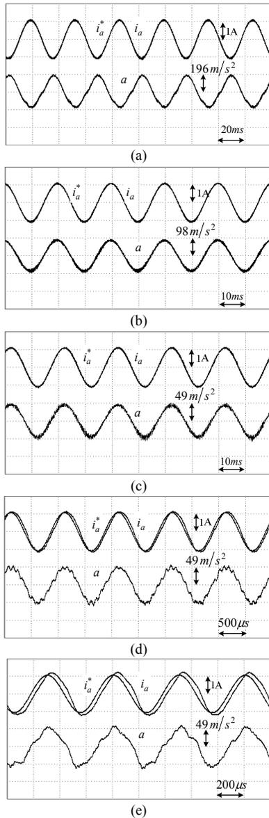
Fig. 12. Experimental results with only feedback loop (load  $0.311kg$ ), (a)  $20Hz/1A$ ; (b)  $30Hz/1A$ ; (c)  $100Hz/1A$ ; (d)  $1kHz/1A$ ; (e)  $2kHz/1A$ .
