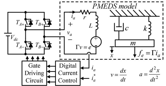
Fig. 2. System configuration and PMEDS model.
