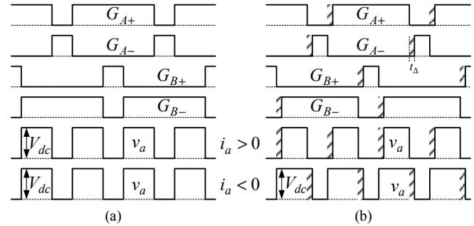
Fig. 5. Gate signals and the resulting armature voltage  $v_a$ : (a) without dead time  $t_{\Delta}$ ; (b) with dead time  $t_{\Delta}$ .
