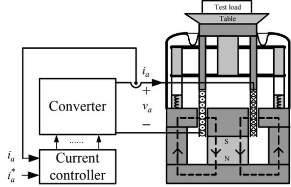
Fig. 1. Permanent-magnet electrodynamic shaker (PMEDS).
