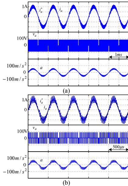
Fig. 9. Simulation results with PI feedback loop and dead-time compensation loop (a)1kHz/1A (no load); (b)2kHz/1A (no load),
