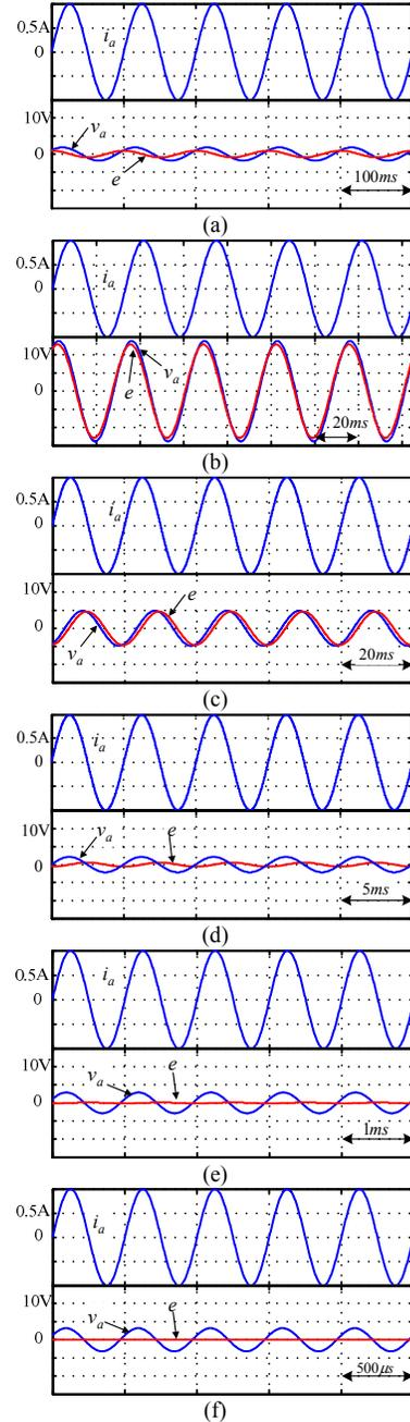
Fig. 3. Simulation no-load results of PMEDS fed by ideal current source: (a) 10Hz/1A; (b) 30Hz/1A; (c) 50Hz/1A; (d) 200Hz/1A; (e) 1kHz/1A; (f) 2kHz/1A.
