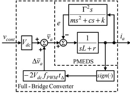
Fig. 6. Equivalent model for full-bridge-fed PMEDS.
